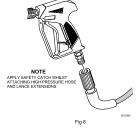
Fig 6. Connect the High-Pressure Hose to the Lance.
